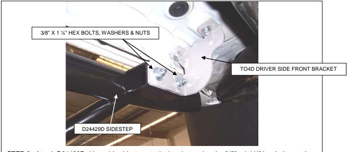
**STEP 6.** Attach D24429D driver side sidesteps to the brackets using the 3/8" x 1 1/4" hex bolts, washers and nuts.
