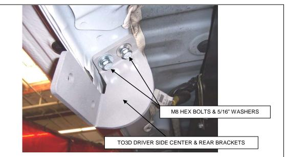
**STEP 5.** Loosely attach the TO3D center and rear brackets, to the body panel using the M8 hex bolts, and 5/16" washers.
