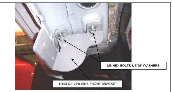
STEP 3. Loosely attach TO4D front bracket to the body panel using the M8 hex bolts, and 5/16" washers.
