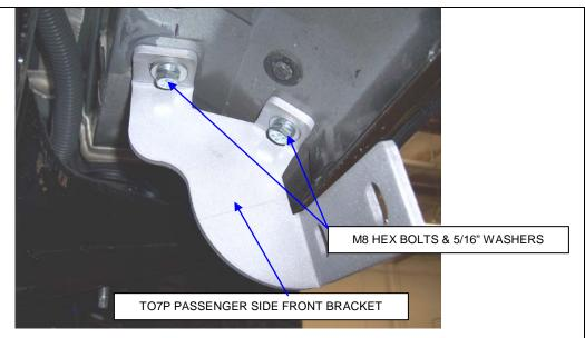
STEP 3. Loosely attach TO7P front bracket to the body panel using the M8 hex bolts, and 5/16" washers.
