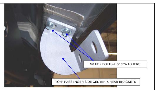
**STEP 5.** Loosely attach the TO8P center and rear brackets, to the body panel using the M8 hex bolts, and 5/16" washers
