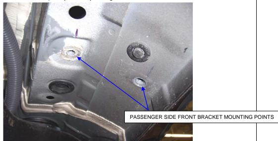
**STEP 2.** This installation uses (3) brackets per side. Begin by installing the passenger side front bracket. Locate the (2) threaded holes in the underside body panel.
