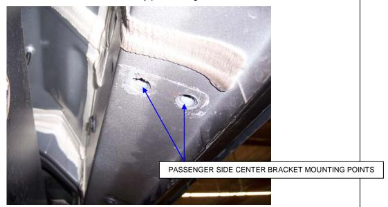
STEP 4. Locate the threaded holes in the body panel, at the center and rear of the cab.
