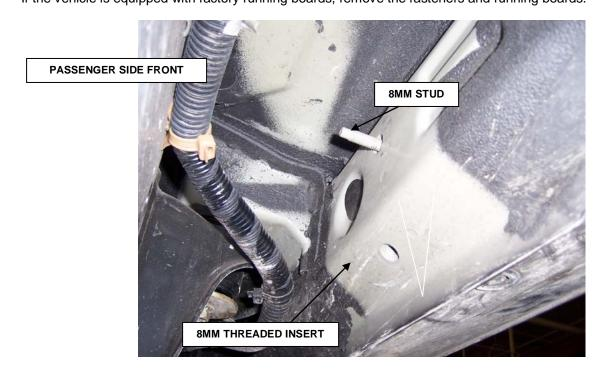
**STEP 2.** This installation uses three mounting brackets per side. Begin by installing the passenger side front mounting bracket. Locate the stud and threaded insert in the under side of the body. Note: you may need to remove the plastic plug to expose the threaded insert.
