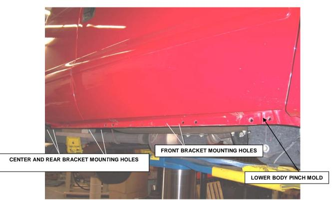
Step 2 This installation uses three mounting brackets per side. Beginning with the passenger side, locate the six
