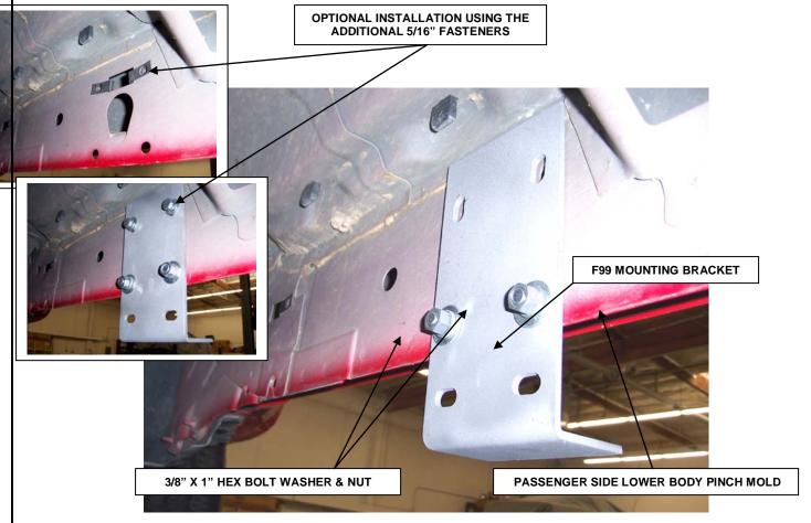
Step 3. Loosely attach the mounting brackets to the lower body pinch mold using the 3/8" x 1" hex bolts, washers,
