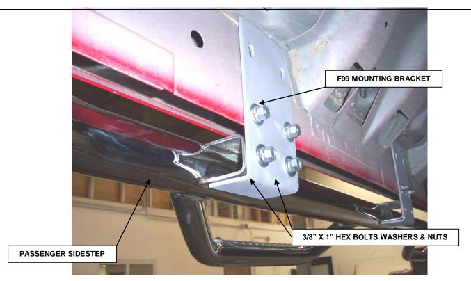
**Step 4.** Position the passenger sidestep up to the mounting brackets and loosely attach it to the brackets using the 3/8" x 1" hex bolts, washers and nuts as shown.
