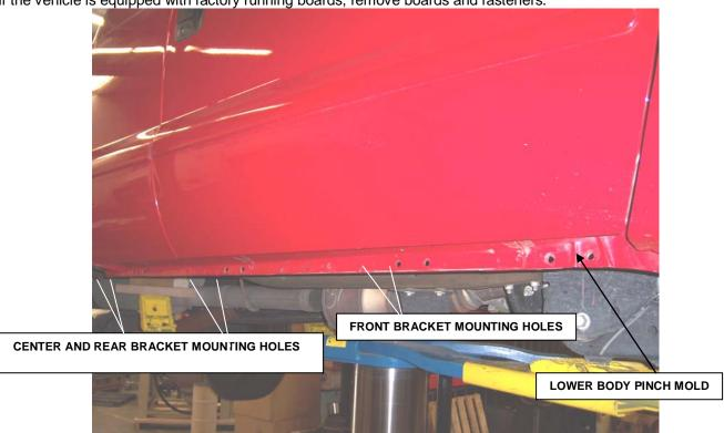
**Step 2.** This installation uses three mounting brackets per side. Beginning with the passenger side, locate the six holes in the lower body pinch mold.
