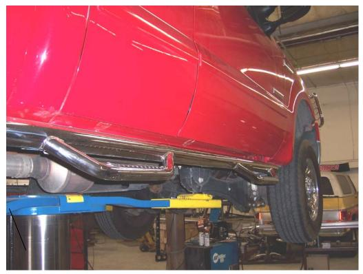
**Step 5.** Align sidestep with the body, and then tighten all mounting bracket and sidestep nuts and **Step 6.** Repeat the above steps to install the driver side mounting brackets and sidestep.
