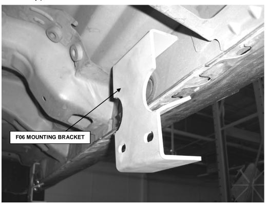
**STEP 6.** Loosely attach the flange of the mounting bracket to the bottom of the lower body pinch mold using the 3/8" x 1" hex bolts, washers, and nuts.
