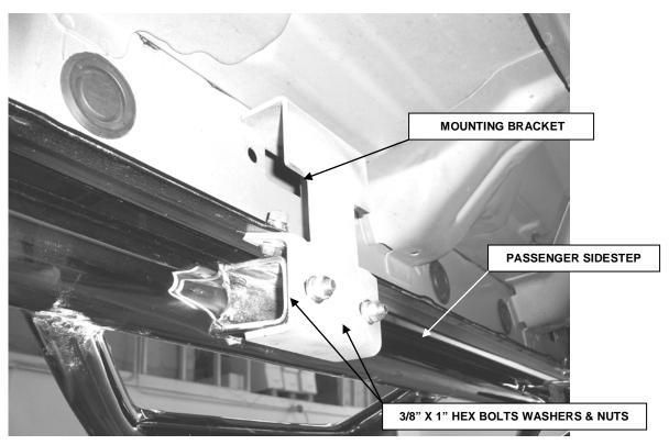
**STEP 9.** Position the passenger sidestep up to the mounting brackets and loosely attach it to the brackets using the 3/8" x 1" hex bolts, washers and nuts as shown.
