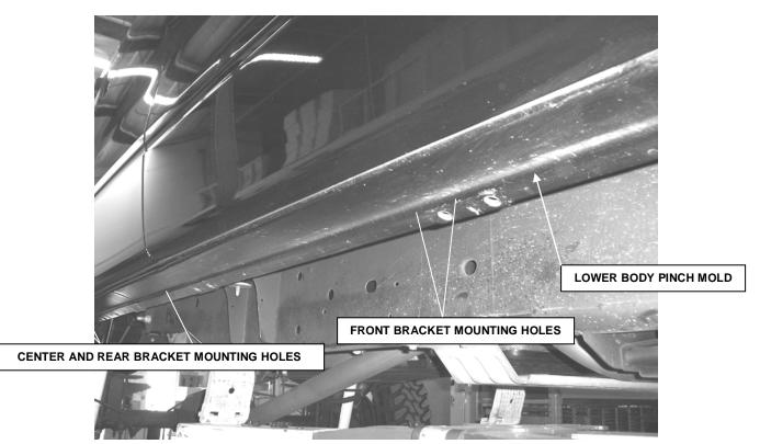
STEP 2. This installation uses three mounting brackets per side.
