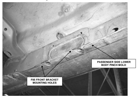
**STEP 3.** Beginning with the passenger side, locate the holes in the lower body pinch mold for the front mounting bracket.
