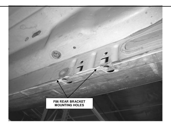
STEP 7. Locate the holes in the lower body pinch mold for the rear-mounting bracket.
