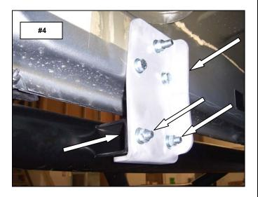
STEP-4 ALIGN THE SIDE STEP WITH THE VEHICLE AND TIGHTEN ALL MOUNTING BRACKET AND SIDE STEP NUTS AND BOLTS. REPEAT THE ABOVE PROCESS TO INSTALL THE DRIVER SIDE BRACKETS AND SIDE STEP.
