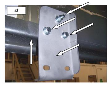
**STEP 2.** ATTACH ONE OF THE MOUNTING BRACKETS TO THE BODY PANEL USING THE T-PLATE (2) 3/8" X 1 ¼" HEX BOLTS, (3) 3/8" FLAT WASHERS, (3) 3/8" LOCK WASHERS AND (1) 3/8" HEX NUT. HAND TIGHTEN. REPEAT THE ABOVE PROCEDURE TO INSTALL THE CENTER AND REAR MOUNTING BRACKETS. **PHOTO'S #2 & #3**
