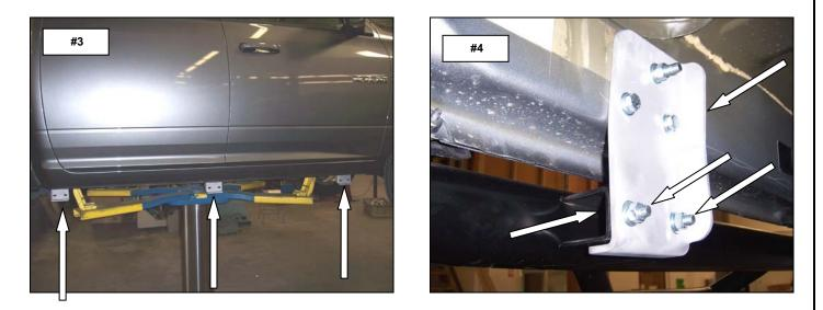
**STEP 4.** ALIGN THE SIDE STEP WITH THE VEHICLE AND TIGHTEN ALL MOUNTING BRACKET AND SIDE STEP NUTS AND BOLTS. **REPEAT THE ABOVE PROCESS TO INSTALL THE DRIVER SIDE BRACKETS AND SIDE STEP.**
