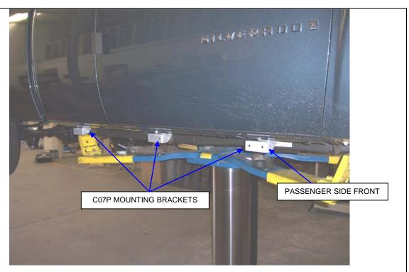
**STEP 5**. Locate the holes in the body for the center and rear mounting brackets. Measure rearward from the front fender bolt 37 ¾" for the center and 67" for the rear bracket. Repeat steps 3 & 4 to install the center and rear brackets.
