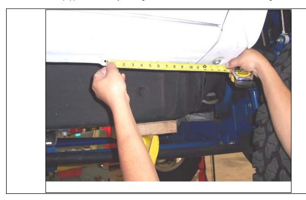
**STEP 2.** This installation uses three mounting brackets per side. Begin by installing the passenger side front mounting bracket. Measure reward from the front fender bolt approximately 14" and Locate the single hole in the body pinch mold and the two holes in the rocker panel.
