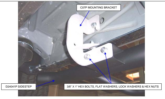
**STEP 6.** Position D24041P passenger sidestep up to the vehicle and loosely attach it to the mounting brackets using the 3/8" x 1" hex bolts, flat washers, lock washers and hex nuts.
