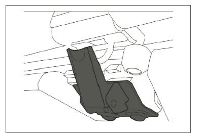
28. Wrap the 2 straps attached to the main section of fabric around the rear-middle of the sound bar. Hook into the holes of overhead brackets. Tighten the strap until snug.
