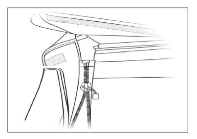
32. Locate the sewn-in plastic strip along the front edge of the Left Side Window.
