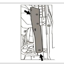
11. Secure the mounting plate to the roll cage using turn-knobs in the holes. Do not fully tighten knob yet.
