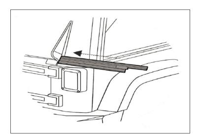
35. Snap the tailgate bar into the mount by pushing the bar against the mounts and rotate tailgate bar downward.
