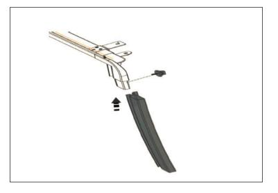
7. Install LH Upright Lower Plastic onto LH Upright and secure with 1 self-tap screw.
