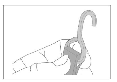
29. Locate the ceiling adjustment straps at the corners of the ceiling panel. Wrap the straps around the roll bar and tub top rail toward the inside of the Jeep, then hook the strap adjust buckle.
