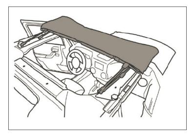
23. Place pivot tubes over the mount hinge plate. Line up the brackets then secure with the counter-sink Allen head screw and nylon lock-nut.
