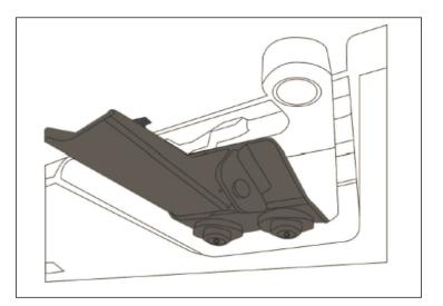
17. Fold back the hardware tubes of the header channel assembly then install the main deck fabric. Secure with snaps as shown.
