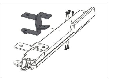
5. Install LH Upper Corner onto LH Rear Door Bar & secure all pieces with 6 self-tap screws.
