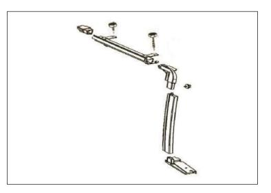
14. Attach the Tailgate Mount to the vehicle rail. Using one OEM Torx head screw. Insert the screw through the retainer, and into threaded holes in the top of the vehicle belt rail, and tighten. Repeat the same step to the passenger side.
