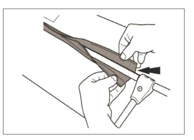
20. Roll up the Soft Top Deck to make installation to the Flip Top Plates more manageable.
