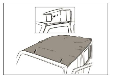
25. Check the front edge to windshield edge lines up to windshield seal.
