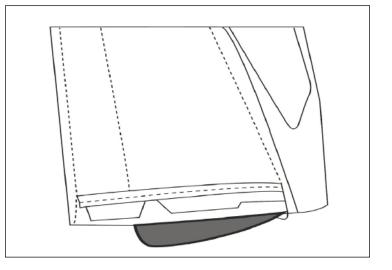
31. Lift up the corners of the top fabric to expose the zippers on the side and rear windows. Secure all windows to the Main Deck by zipping fully into place.
