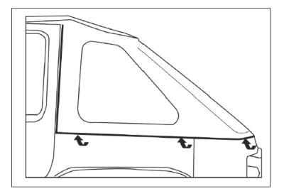
34. Slide the tailgate bar onto the bottom of the rear window.
