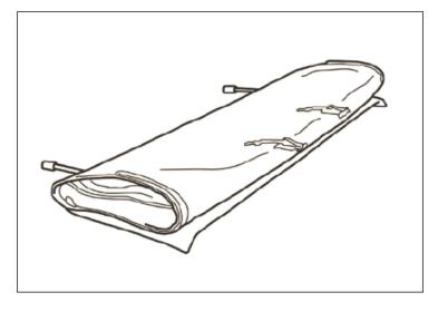
22. Lift the soft top and header channel assembly onto the windshield gasket.
