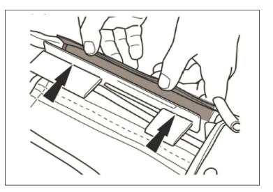
19. Secure the Flip Top Header Assembly to the Soft Top Deck by engaging the Hook and loop flap around the tube.
