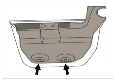
16. Place provided latch as shown and reattach with the screws from the previous step. Do not tighten the screws and adjustment may be needed. Repeat steps 17-18 for the other side.
