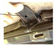
S tep (3): R elease the rear corners of the top. Pull gently down and then out to release the plastic strip from the retainer on the vehicle.
