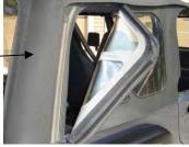
Step (2): Release the front of the top from the windshield. Raise the front of the deck and collapse the rear bows, tucking the two plastic strips above the door opening and the stay pad on the rear bow inside of the bows. Wrap the fabric around the bows, then tuck the rear legs of the top under the bows.
