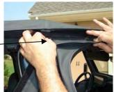
Step (9): R oll the plastic along the front of the panel into the channel of the door surround on the vehicle.
