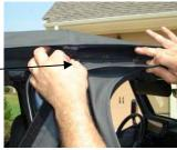
**Step (9):** Roll the plastic along the front of the panel into the channel of the door surround on the vehicle.
