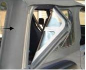
Step (2): Release the front of the top from the windshield. Raise the front of the deck and collapse the rear bows, tucking the two plastic strips above the door opening and the stay pad on the rear bow inside of the bows. Wrap the fabric around the bows, then tuck the rear legs of the top under the bows.
