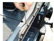
Step (3): Flip the fabric over so that it wraps around the header and drape the top fabric over the tailgate. Raise the header slightly and work the pockets in the fabric over the corners of the header. Install an oval head screw in each corner to secure the fabric to the header.
