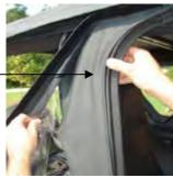
**Step (10):** Locate the plastic strip sewn to each side of the top, above each door. Slip the strips into the channel in the door surround above the door opening.
