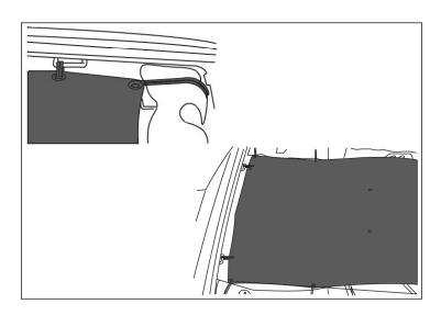
6. Pull the top all the way back and attach the rear strap to the hole in the back of the roll bar. Tighten the strap until snug.
