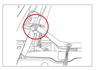
5. Tighten and adjust as needed to be centered on top of the roll cage.
