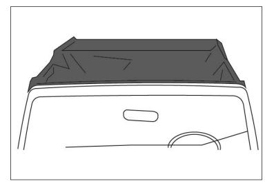
2. Tuck inside and secure with bungee straps as shown.
