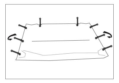
3. Secure with bungee strap around roll cage as shown.
