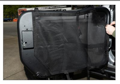
5. Secure Mesh Cover by looping straps around tube. DO NOT fully tighten at this time.
