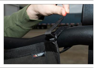
6. Slide Tube Door check strap through cutout in the Mesh Cover and attach check strap to Tube Door.
