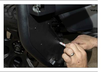
3. Attach cut Loop Strips to back of Tube Door, as shown.
