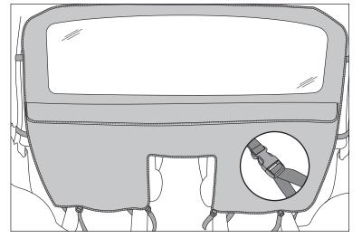
5. Zip windbreaker to tonneau cover using zipper under flap of windbreaker.
