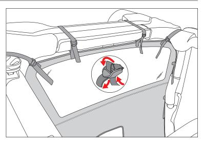
3. Thread side straps loosely around side sport bars as shown.
