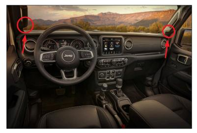
2. Insert the long button head bolt with flat washer through the side mount and thread into the windshield pillar threaded hole that was left from the bolt removed in step 1. Do not fully tighten at this time.
