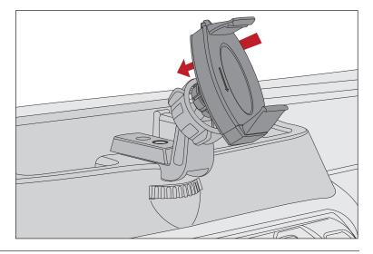
3. Pull Outer Ring over Phone Mount adapter and twist to secure.
