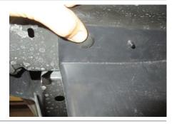
Remove the two factory bolts in the bottom of the frame using an 18mm socket. Next, remove the two factory bolts securing the rearward exhaust hanger bracket with a 10mm socket.
