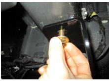
Torque all M12 fasteners to 79 ft-lbs. and all 7/16" fasteners to 59 ft-lbs.
