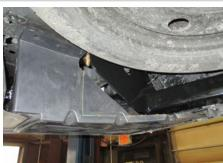
Raise the exhaust back into position and reattach the three rubber hangers. The rearward most rubber hanger will be secured to the post on the hitch.
