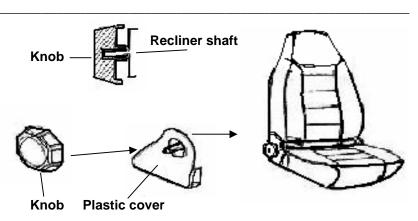
Step (1) Firmly press plastic cover to the side of the metal seat recliner bracket for each side.
