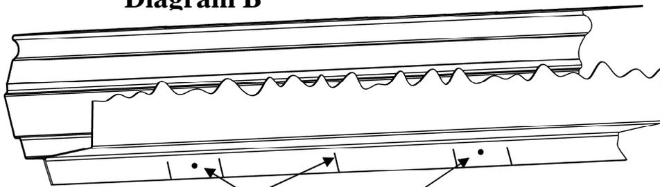
Marked vertical line that was transferred from Diagram A to the inside of the rocker panel.
