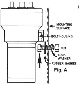
1. Install the compressor in the engine compartment in a dry location and safe from engine exhaust manifold heat. To secure the compressor, drill a 3/16-inch hole through metal and mount compressor vertically (air outlets at the top). Insert head of bolt into the bolt housing and secure to the vehicle referring to Figure A. Use mounting hardward in the order shown – bolt, rubber gasket, mounting surface, lock washer, nut.
