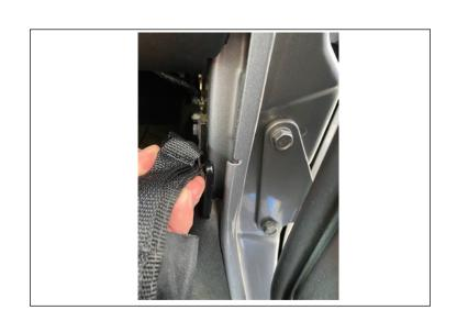
3. Remove T30 Torx bolts from footman loop securing strap to door. Remove footman loop from OE strap.
