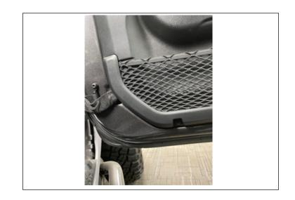
7. Slide desired loop back onto factory retainer hook and reconnect door harness.
