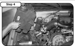
Lift up and remove the airbox assembly.
