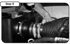
Place the supplied coupler and clamps on the air filter. Secure the MAF sensor and tighten all the
