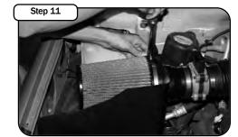
Install the pre-oiled air filter in the housing and secure with the supplied clamp. Do not use any grease or oil.
