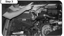
Diconnect and loosen the clamp on the MAF sensor (1). Remove the three 10mm bolts securing the air box. Disconnect the Temp sensor located on the side of the air box.
