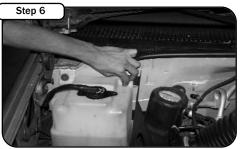
Place housing in engine bay. Secure with the bolts removed in step 5. Rear housing tab slips in behind plastic.
