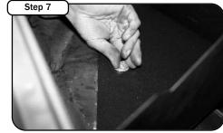
Re install 7/8"mm bolt in the bottom of the housing. Insert bolt thru the fenderwell and secure with supplied lock nut and washer.
