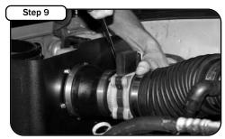
Place the supplied coupler and clamps on the air filter. Secure the MAF sensor and tighten all the clamps.
