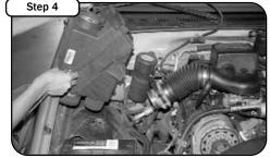
Lift up and remove the airbox assembly.
