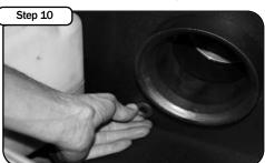
Slide the supplied grommet in the side of the housing. Install the Temp sensor.
