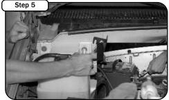
Loosen 10mm bolt on side of coolant reservoir. Remove airbox bracket from inner fender panel. Remove 10mm bolt near batter tray.
