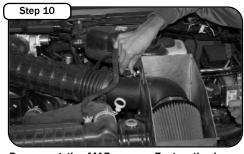
Reconnect the MAF sensor. Fasten the lower air box clips to the new housing.
