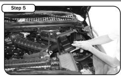
Remove the air box and factory air filter.
