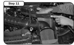
Place the trim seal along the edge of the housing. Start at one end and work you're way around the edge.
