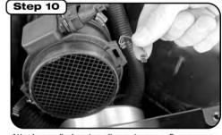
Attach supplied spring clips onto mass flow sensor insert hooked end into slotted section on mass flow sensor.
