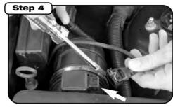
Remove mass flow sensor plug and hose clamp (1/4" nut driver)
