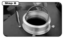
Install the billet aluminum adapter to the shield. Use the M6 button heads supplied.
