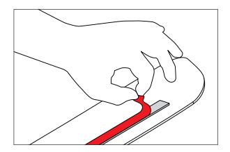
5. Attach rocker guard to the vehicle keeping part aligned to the vehicle surface. Apply pressure to ensure a strong bond. Tighten bolts and nuts.
