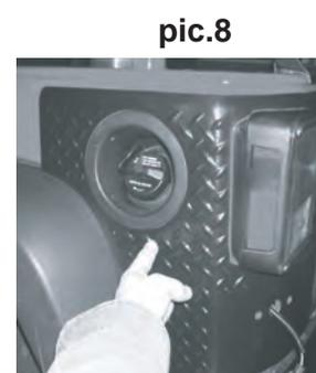
**Step8:** Place Corner Armor into position. The cover will slip over the rear taillight and onto the body of the vehicle. DO NOT remove tape at this time. Visually inspect the fit of the part to confirm that the gas filler neck cover and license plate mounting holes are aligned. Confirm the cover matches the body contour and shape. You may trim the armor where needed (pic.3).
