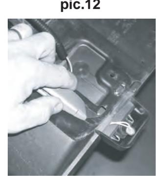
**Step11:** Pull protective covering from behind cover. DO NOT apply pressure to the cover until all protective strips have been removed. Check fitment one more time before applying pressure to the remaining tape sections (pic.10).
