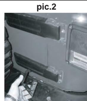
**Step2:** Remove the two plastic tailgate hinge covers located on the right rear corner of the vehicle (pic.2).
