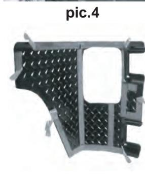
**Step4:** With the Rear Armor removed from the vehicle peel back 2" of the outer edge protective covers at 45 deg. angles. All inner protective covers should be removed (pic.4).
