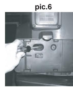
**Step6:** The removal of the rear license plate holder is required for the installation of the left side Corner Armor. After removing license, unbolt the 4 small 8mm screws holding the license plate holder to the body (pic.6).
