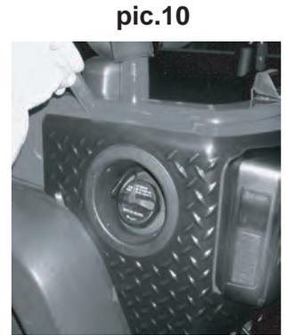
**Step10:** Place Rear Corner Armor back over rear taillight being careful not to touch the body with the exposed 3M tape. With the Corner Armor aligned to the fill neck opening affix sections of exposed tape making sure that the cover is flush. Double check to the vehicles body contours. When positioned correctly apply pressure working from the filler neck around rear corner to tailgate.
