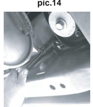
**Step14:** Bumper should pull back and off vehicle. After corner armor has been attached and the license plate holder secured reinstall rear bumper to vehicle.
