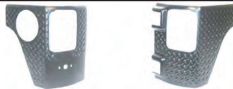
**Note: The Wrangler body armor has been designed to fit tightly to the contours of the vehicle. Instructions must be followed to insure the correct placement and adhesion of this part. If surface is not cleaned and prepped as stated in the instructions proper fitment will not take place. Do Not install if outside temperature is below 65F. or over 100F. Allow part to sit overnight before driving.**
