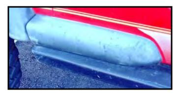
Flare extensions can be reinstalled, but holes will need to be drilled in side rocker armor after they have been installed.
