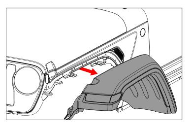
2. Using a clip removal tool or pry tool, remove any plastic clips still on fender. Thoroughly clean exposed fender.
