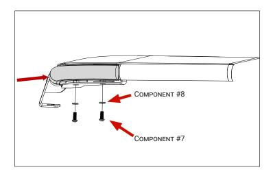
6. Position tube flare on vehicle. Using supplied M8 hardware, loosely attach flare to the OE mounting tabs.
