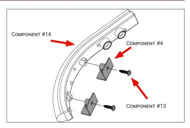
5. Position light and light brackets in the cutout in the flares. Using the supplied short button head bolt and M6 washers, loosely attach light brackets to tube flares.
