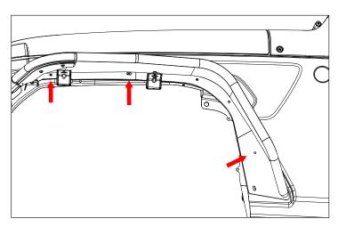
8. Using M6 lock nut(#5), M6 Large O.D Washer(#9), long button head bolt(#6), loosely attach tube flare to vehicle.
