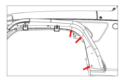
9. Connect the wire harness for the running/indicator light to the OE plug. Zip tie wires and control box to fender taps. Tighten all hardware. Repeat this process on the opposite side. Reconnect primary and secondary batteries.
