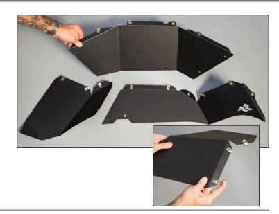
2. Attach the center and rear panel together using 20mm Allen head bolts and washers. Don't fully tighten at this time.
