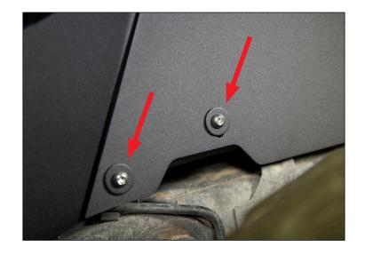
6. Completely tighten all hardware. When tightening make sure the panel does not bind or pitch any wires or lines.
