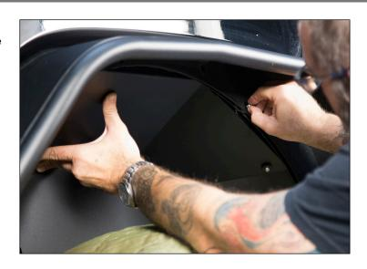
5. Two 35mm allen head bolt use washers and ny-lock nuts instead of threading into U-clips.
