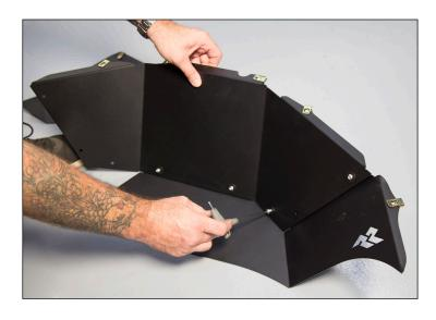
3. Attach the front panel to the other two panels from step two. Use 20mm allen head bolts and don't fully tighten at this time.
