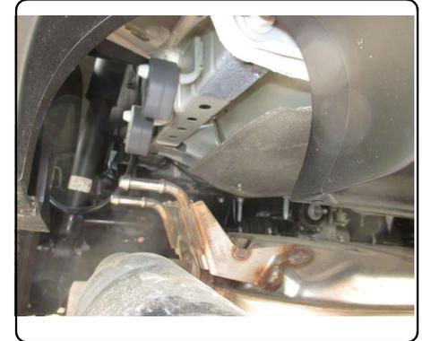
2. Using a die grinder, enlarge the third from the back of the vehicle bottom hole in the frame as needed to fit the supplied spacers and carriage bolt heads. (both sides) If excess sealer is in the mounting holes, remove with a utility knife.
