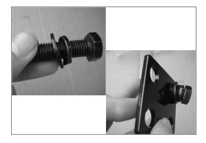
5. Remove the bolt that was installed in step 2. Rotate the backing plate so all of the holes line up with the holes in the sub-frame. Thread another bolt and washer assembly into the top right corner of the backing plate and sub-frame into the tow hitch.
