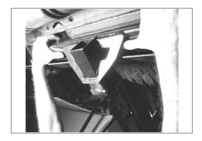
2. It is necessary to temporarily locate and secure the tow hitch in order to ease the installation of backing plates. While supporting the tow hitch thread a supplied M12 bolt through the top right corner of the sub-frame and into the corresponding welded nut of the tow hitch.
