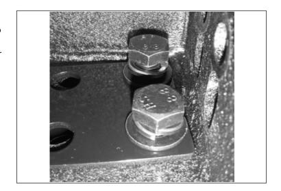
6. Install 2 more bolt and washer assemblies through the backing plate, sub-frame, and into the tow hitch. Do not tighten the bolts at this time.
