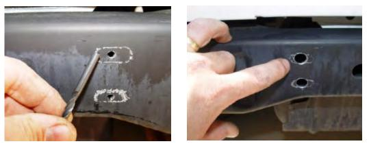
Attach the hitch with the (4) 10mm bolts, flat washer, lock washer and nuts supplied for each side. Tighten to 45lbs (Total of 8). **NOTE: ON 97-2006 Wranglers there might be a tight fit between the rear cross member and the fuel tank. A second person will help with installation.**
