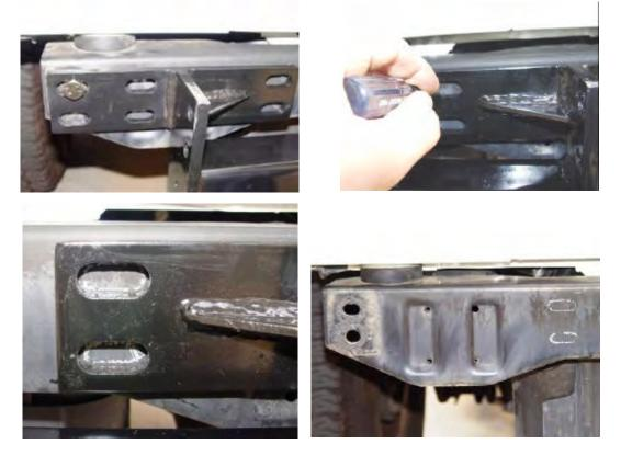
Step (3)Drill holes into rear cross member.WARNING ... BE VERY CAREFUL WHEN DRILLING<br/>MOUNTING HOLES. THE FUEL TANK IS LOCATED JUST BEHIND THE CROSS MEMBER.<br/>Great care will be needed to avoid puncturing the fuel tank.<br/>Use a small 3/16" drill bit for a starter hole. After the small holes have been drilled, enlarge<br/>them with a 1/2" drill bit. BE VERY CAREFUL TO AVOID HITTING THE FUEL TANK WHEN<br/>DRILLING.
