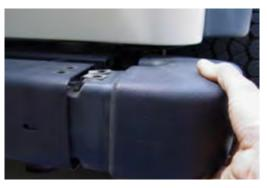
For some 97-2006 Wranglers the rear body mount and bolt may need to be removed to gain access to the top inside rear bumper bolt.
