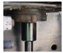
Step (2) Align inner and outer mounting holes with the rear frame cross member. (2 outside of frame rail, and 2 inside frame rail for each side).
