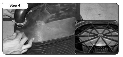
Re-assemble the air filter assembly. Verify engagement grooves are positioned as shown to ensure correct installation. Reinstall assembly back into engine.
