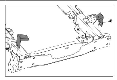
7. Position Bumper Shell and Tow Hooks into place on vehicle's frame rails. Using supplied M12 hardware and Nut Plates, loosely attach Bumper Shell and Tow Hooks using center four holes.
