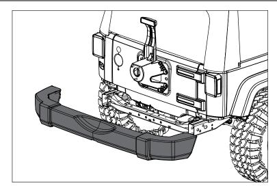
2. Install Left and Right Mounting Brackets into frame rails using Hex Head M12 Bolt, Lock Washer, and Oversized Washer. Do not fully tighten hardware.
