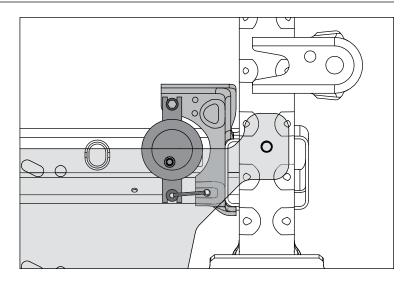
12. Remove fog lights from factory bumper and install on Spartan Front Bumper using supplied M4 hardware.
