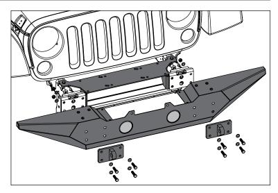
15. Fasten Spartan Front Bumper to Winch Plate using supplied M8 hardware. Tighten all fasteners and reconnect fog lights.
