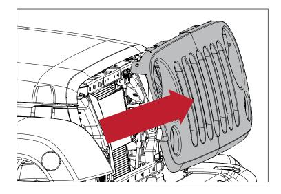
5. Remove factory plastic closeout panel by releasing the plastic fasteners that attach to each frame rail.
