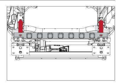
6. Unbolt and remove factory vacuum pump. Retain factory bolts.
