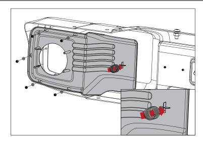
4. Remove bulb from factory fog light housing and install housing to bosses in Plastic Cover using supplied Thread Forming Screws. Do not overtighten.
