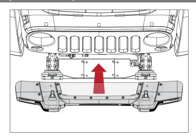
28. Place Stanchion, Bumper Mount Bracket, and factory Tow Hook on frame horns and secure with OE Nuts. If not using Tow Hooks, replace with M12 Hex Head Bolts and Lock Nuts.
