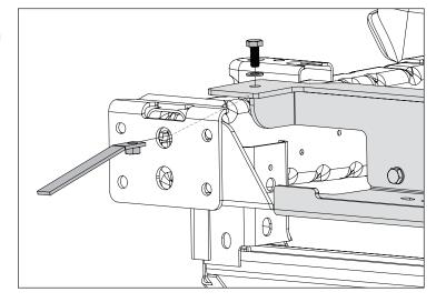
22. Insert Support Bracket into opening in frame and secure with supplied M12 Hex Bolts and Flat Washers.
