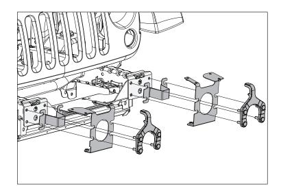
29. Position Bumper Center Section to accept factory tow hooks and lower into place on frame rails. Align with holes in Bumper Mount Brackets and secure with M10 Button Head Bolts, Plastic Flat Washers, and Hex Nuts. Tighten bolts attaching Bumper Mount Bracket to vehicles frame.
