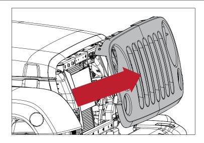
11. Remove factory plastic closeout panel by releasing the plastic fasteners that attach it to each frame rail.
