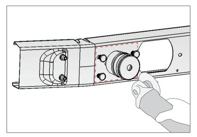
25. Insert Tow Hooks into opening in Bumper Center Section. If not using Tow Hooks, replace with M12 Hex Head Bolts. Place Crush Can and Bumper Mount Bracket in place in front of Tow Hooks or M12 Bolts.
