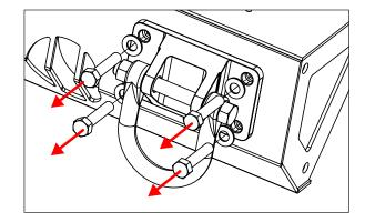
2. Align new Welded D-Ring Bracket and fasten to bumper as shown using supplied M12 hardware.
