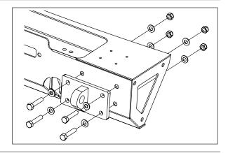
NOTE: For custom applications, drill four 1/2 inch holes using Welded D-Ring Bracket as template.
