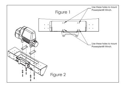
3. Once all 4 Winch bolts have been started, tighten them. Installation of the Winch and the Winch Spacers is now complete! Proceed with the remainder of the installation as demonstrated in the main Bumper Installation Instructions.
