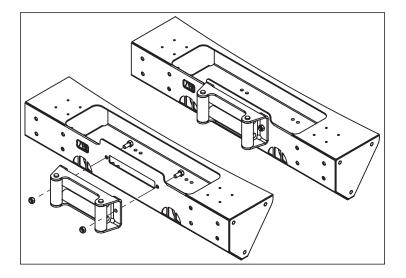
2. Prepare Winch and vehicle for installation as specified in winch installation instructions. Align holes in bumper as shown below (Figure 1) with Spacers and winch mounting holes (Figure 2). It may be helpful to thread winch cable through Fairlead before bolting it in place. Install winch as instructed by winch manufacturer, but substitute standard bolts supplied with the winch for longer bolts supplied with the spacers.
