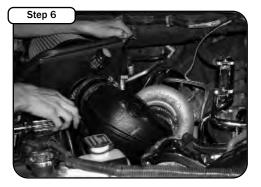
Tighten all the clamps snug but do not overtighten.
