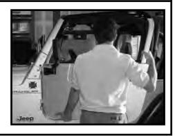
4. To install Tube Doors, lightly lubricate the tube door hinge pins. Position the hinge pins directly above the hinges. Slowly lower the hinge pins into the door hinges. If the hinge pins do not fully seat, slowly rotate the door back and forth until hinge pins fully engage. Install OE nuts removed in the previous step.
