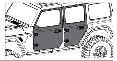
2. Loosely install Hinge Pins on Tube Doors using supplied M8 hardware.
