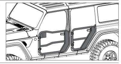
4. Close Tube Door and tighten Hinge Pin hardware. Install Check Strap using shortest setting. Cycle Tube Door open and closed to ensure Hinge Pins are properly aligned and fully seated in door hinge.
