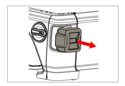
3. Unplug tail light by sliding red tab first. Then press down on gray tab and gently pull plug from light.
