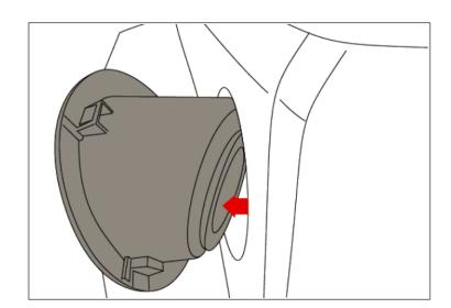
6. Align grommet on filler housing with fuel filler neck. Apply moderate pressure to front face of fuel door to engage.
