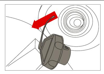
5. Remove OE fuel filler housing, by releasing plastic tabs on back of fuel housing. Pull fuel filler housing to remove. Clean area previously covered by filler housing before proceeding.
