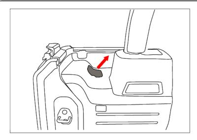
2. Using either a 10mm or T40 torx socket, unscrew OE mounting bolt and carefully pull tail light away from vehicle.
