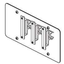
Attach Hawse Fairlead License Plate Holder to Hawse fairlead by aligning the 3 snap fittings with the opening in the fairlead. Route winch line between the snap fittings and push the plate evenly until fittings engage. Use supplied License Plate Mounting Bolts to attach license plate.
