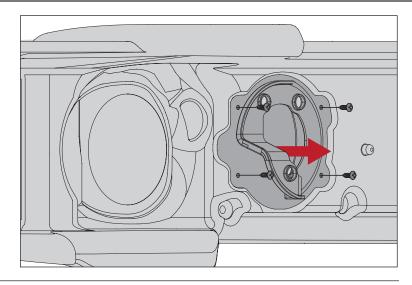
2. If using O-Ring, place around outside of Guard.
